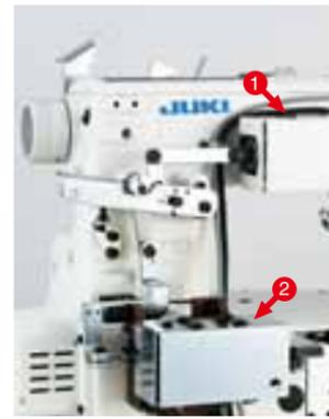
① Presser lifter drive mechanism magnet
