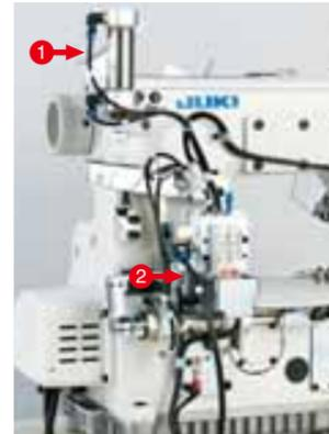
① Presser lifter drive mechanism air cylinder
