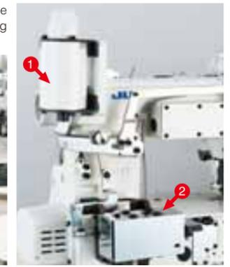
① Presser lifter drive mechanism magnet
