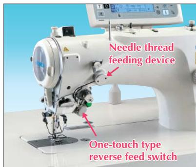
Troubles are prevented at the beginning of sewing by keeping the bobbin thread tension low
